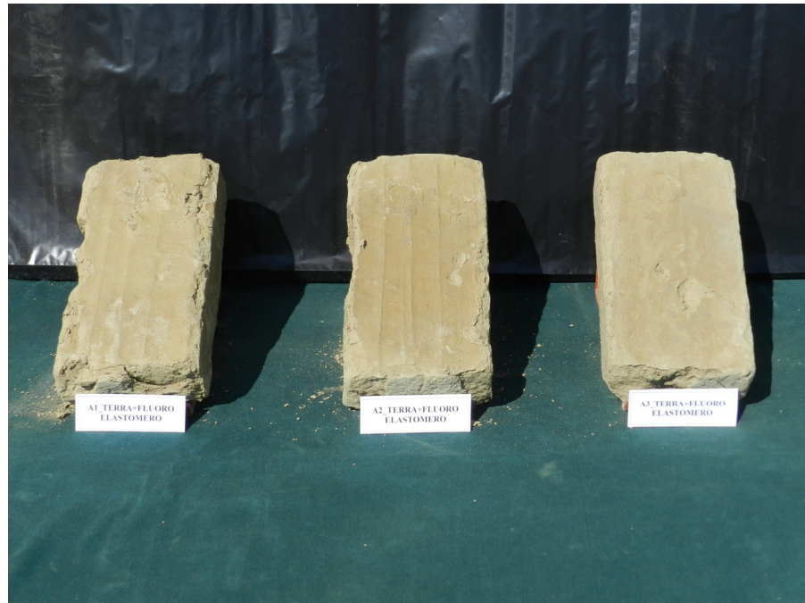
Figure 5. Earthen bricks: Specimens made with local earth (from Alessandria, Italy) and treated with a fluoroe elastomer (Tecnoflon N215).
