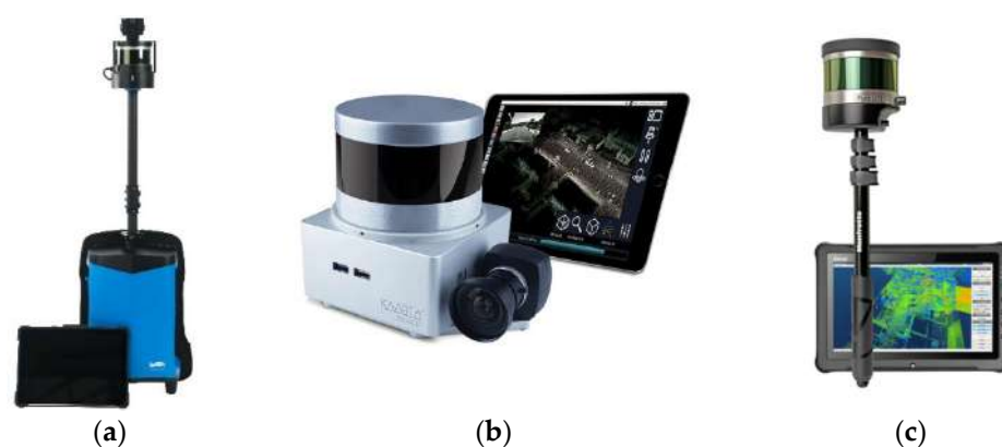
Figure 4. The three tested MMS: LiBackPack C50 (a) Kaarta Stencil (b) and Gexcel Heron Lite (c).
