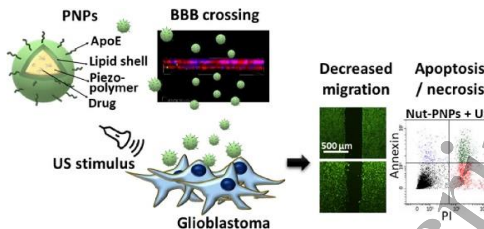
Figure 2. Piezoelectric hybrid lipid-polymeric nanoparticles, composed of the piezoelectric polymer poly(vinylidene fluoride-trifluoro ethylene) and of a lipid shell of 1,2-distearoyl-sn-glycero-3-phosphoethanolamine-N-[amino(polyethylene glycol)], encapsulating the non-genotoxic drug, nutlin-3a, and functionalized with a ApoE-derived peptide, that enhances the BBB crossing abilities of the nanoparticles. Upon ultrasound stimulation, the nanoparticles were able to reduce cell migration, thanks to a reduce f -actin/ g -actin ratio, and to foster apoptotic and necrotic events (Reproduced from [6], Copyright 2021, with permission from Elsevier).
