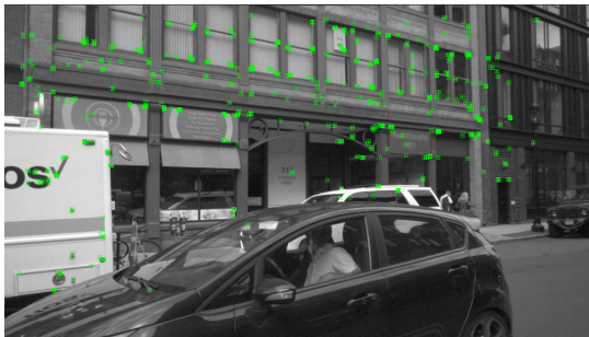
Fig. 3. Example of a scene in which the CAM_BACK_RIGHT fails due to the high number of moving objects (cars) present in the field of view.
