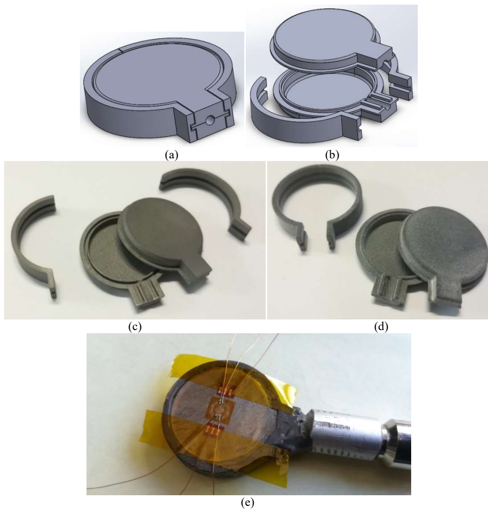
Fig. 1 Drawing of the capsule samples in the assembled design configuration (a) and exploded view (b). Samples parts after AM fabrication process in Ti6Al4V (c) and grey PA (d) and sample with strain gauge during the steps of sensor application (e).
