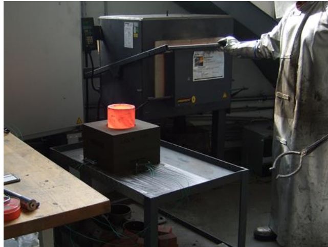
Figure 13: F-TPS finished sample during thermal test, [2].
