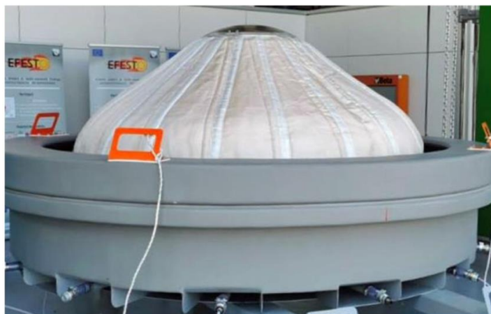
Figure 14: IAD with integrated F-TPS positioned in static deflection test pool, [3].
