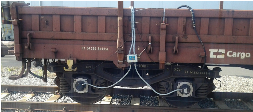
Figure 3: Monitoring system installed on the freight test vehicle in Velim.
