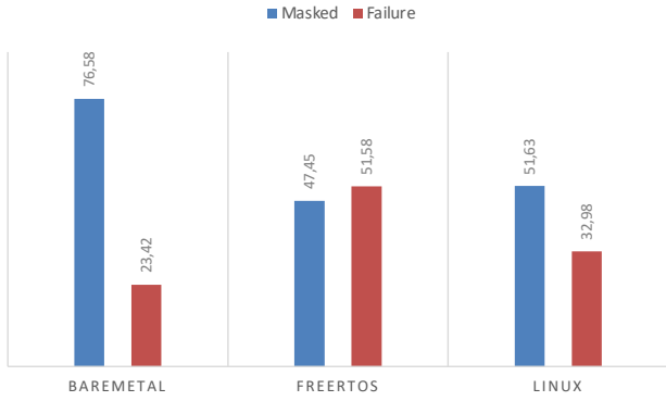
Fig. 2. OS impact of failures
