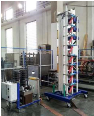
Fig. 2. LATFC's Haefely Impulse generator.
