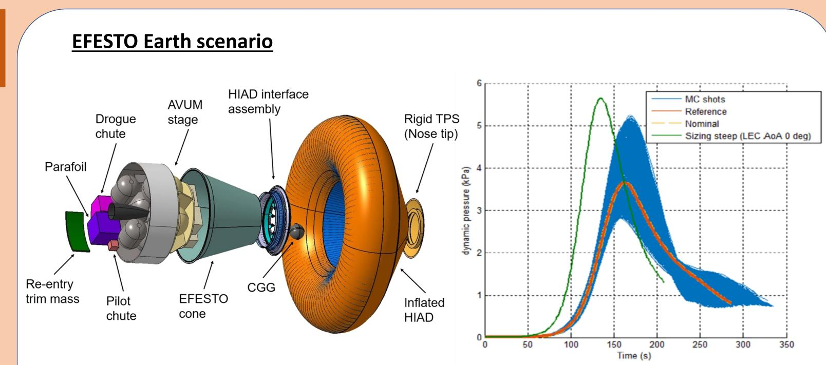
System configuration and sizing dynamic pressure profile
