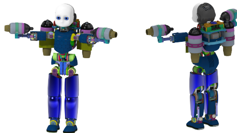
Fig. 1. iRonCub: the jet-powered humanoid robot. The jets are attached to the arms and the chest and exert 160 N and 220 N respectively.
