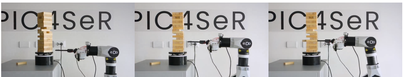
Figure 1. Our proposed solution in action: from left to right in the sequence, the e.DO robot selects a block to extract in the tower, adopting a visual-based control to approach it. Then, it starts pushing for the block extraction if it detects a low reaction force.
