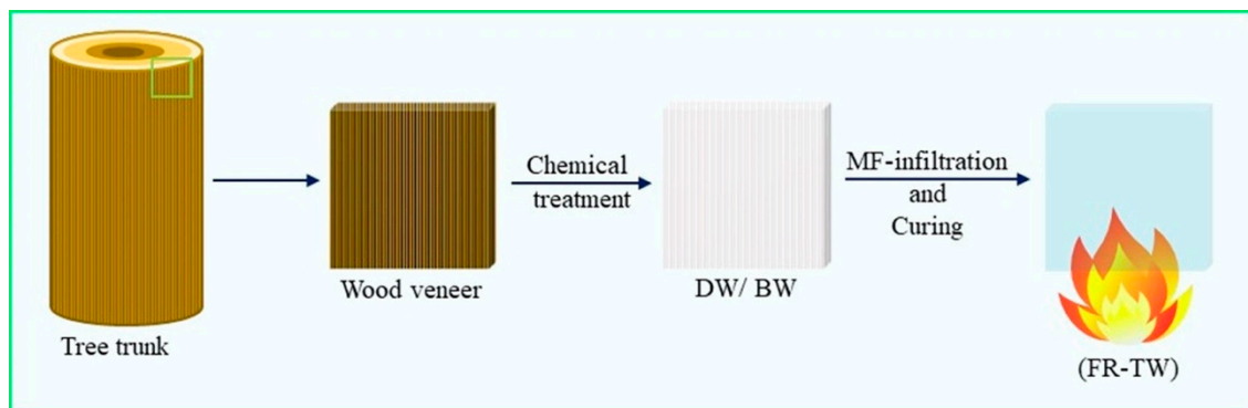
Figure 37. Schematic illustration of fire-retardant transparent wood (FR-TW) fabrication based on melamine formaldehyde, MF. DW is delignified wood where most lignin is removed, and BW is bleached wood where lignin chromophores are modified and a small amount of lignin removed. Reprinted from [50] under CC-BY license.
