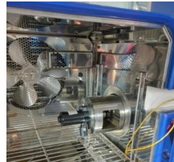
Fig.7 The slender PM motor inside the climatic chamber.
