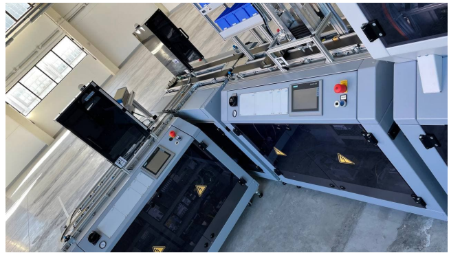
Fig. 3. CP-Factory, a smart and modular assembly line by Festo.
