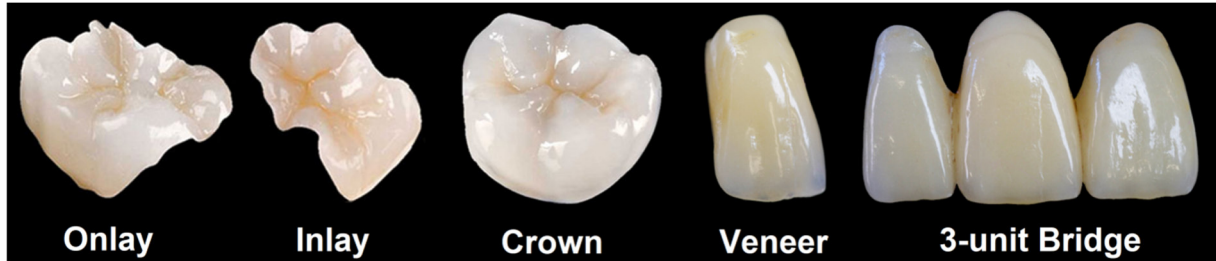
Figure 6- Images of restorative dental glass-ceramics [16,62].
