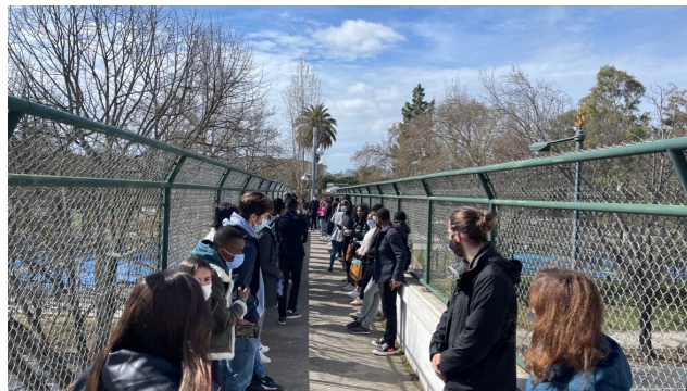
Fig. 4.9 Ambient vibration test on Bridge A with additional mass caused by pedestrians.
