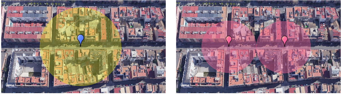
Fig. 2.4 Map of the geographical area served by the EVS service, featuring two intersections and including an IEEE802.11p RSU: one EVS instance and corresponding covered intersections highlighted in yellow (left), two EVS instances and corresponding covered intersections highlighted in pink (right)
