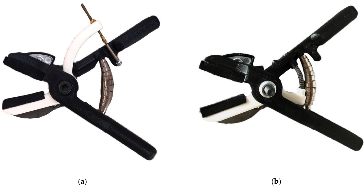
Figure 5. First prototype assembled in two configurations: with traction spring (a), with compression spring (b).
