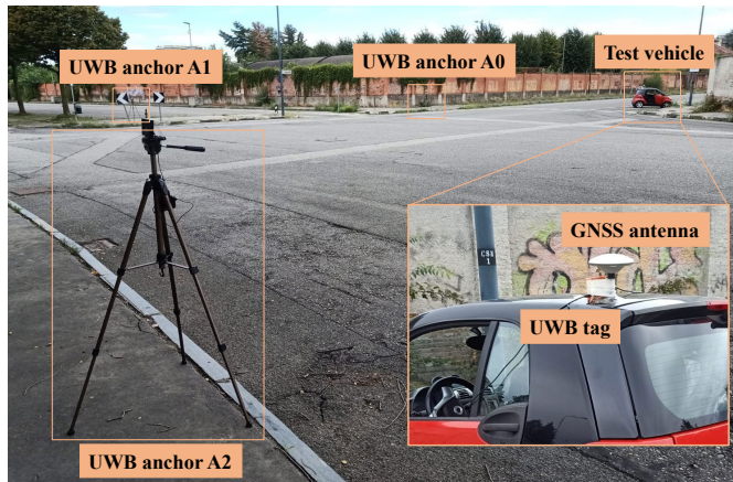
Fig. 11: Snapshot of the experimental scenario for the real-world test campaign. The deployed network of static UWB anchors is shown. Moreover, the UWB tag and the GNSS antenna on the road vehicle's roof are highlighted.
