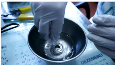
Fig. 5. Grease removal process from the bearings.
