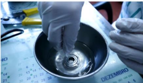
Fig. 5. Grease removal process from the bearings.
