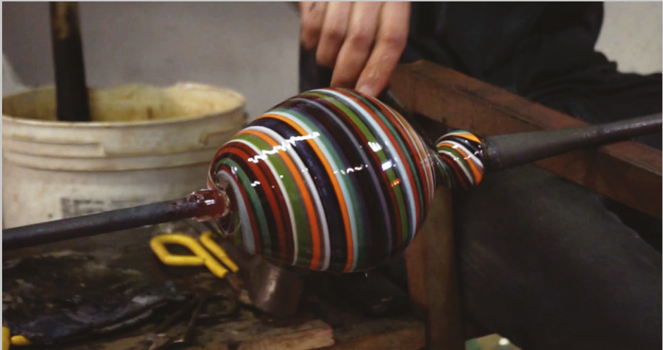
Fig. 01 Joga Glass workshop. On the table, combinations of glass rods prepared to be heated and picked-up with the roll-up technique.
