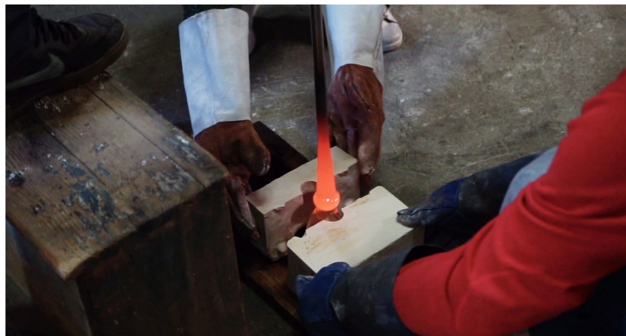
Figure 5. Two students collaborating to remove the blown object from the mould. Particular precautions must be taken during this step as the material is still extremely hot and delicate.
