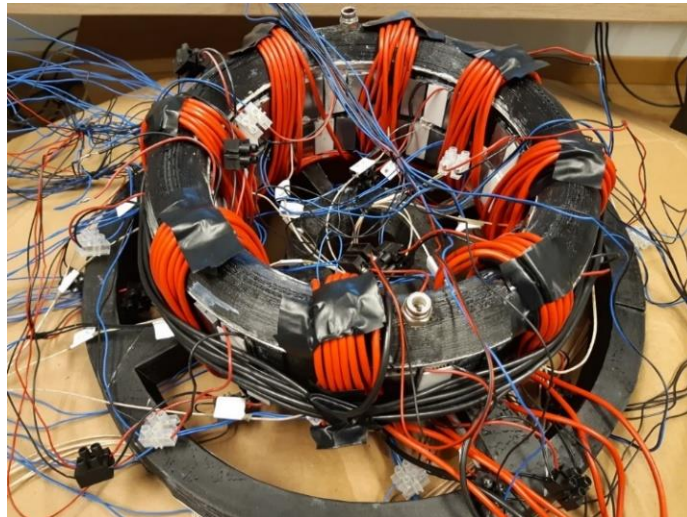
Figure 49: TORODYNA prototype in operating conditions with poloidal coils.
