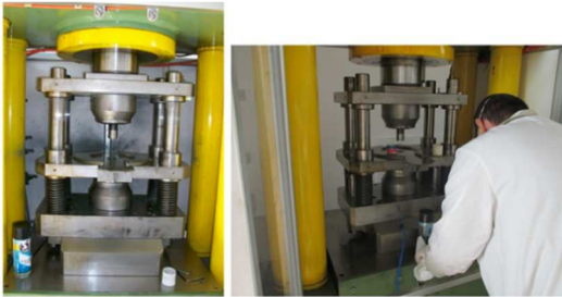
Fig. 5. 200 tons press adopted to realize the specimens
