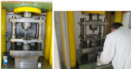
Fig. 5. 200 tons press adopted to realize the specimens
