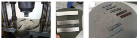
Fig. 11. Sample in the form of a parallelepiped for Single Sheet Test
