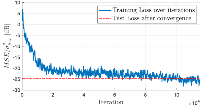
Fig. 5. Evolution of the loss function (i.e., MSE normalized with respect to \bar{y}_{adc} power) over training iterations. Blue curve: training loss over iterations; Red dashed line: test loss after model convergence. Training and test sequences are relative to the qualitative analysis illustrated in Fig. 4
