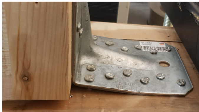
Figure 5: View of the angle bracket tested by the authors.
