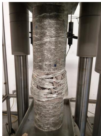
Figure 1 - Failure of GFRP on a reinforced concrete circular column
