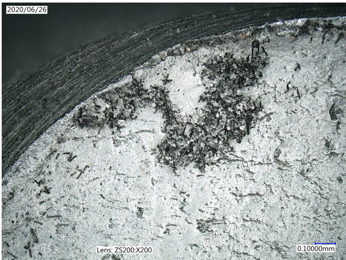
Figure 1 Microstructure of defect in additively manufactured AlSi10Mg
