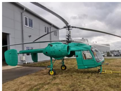
Figure 1 – The demonstrator of SHM based on operating helicopter
