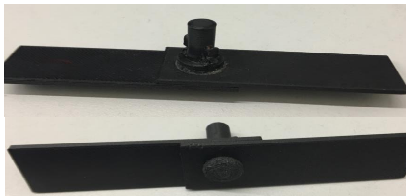
Figure 1 – FSSR specimen for joining 30% short glass fibre composite
