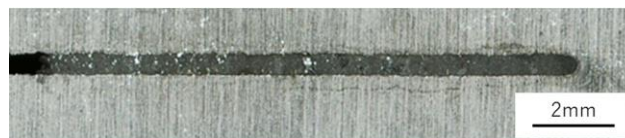
Figure 1 – Optical microscopy result of a simulated crack of the aging-repair specimen.
