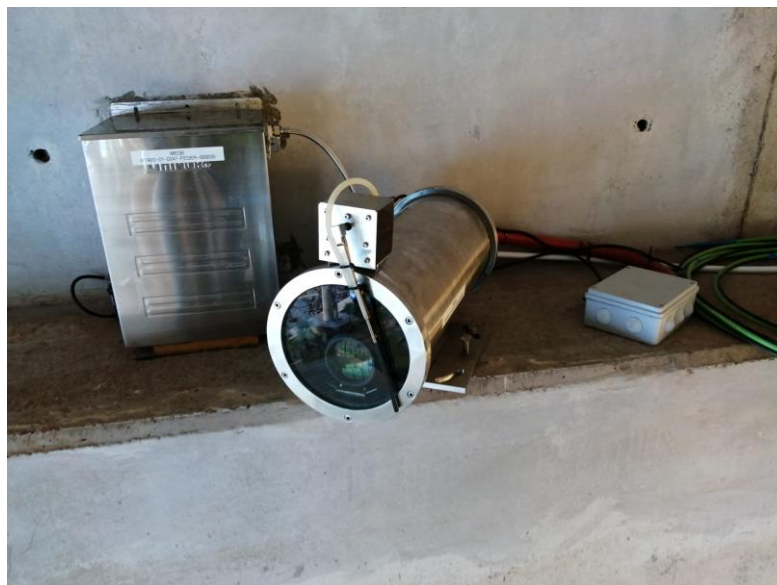
Figure 1 – Image acquisition system installed above one of the pillars supporting the runway
