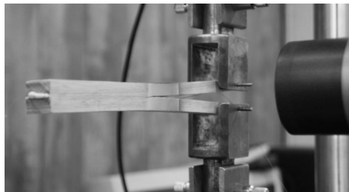
Figure 1 – DCB set-up coupled with DIC
