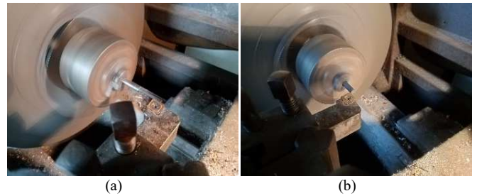
Fig. 18 - Removal of front (a) and side (b) roughness
