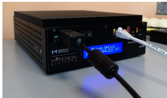
Figure 3: Luna's Micron Optics HYPERION si155 is used as interrogator.
