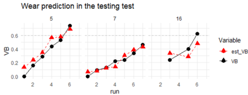
Fig. 4.15 Comparison between test data and estimated values by NN for wear
