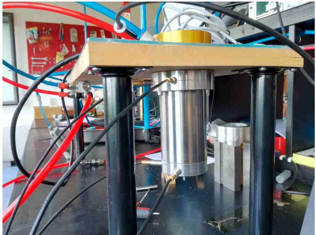
Figure 1. The electro-spindle under test.
