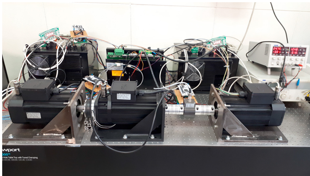
Fig. 3: HIL mechanical bench overview
