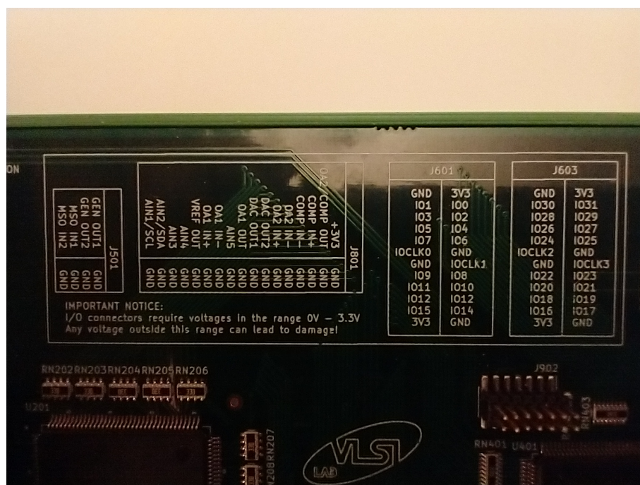
Figure 8. Legend of external I/O connections.
