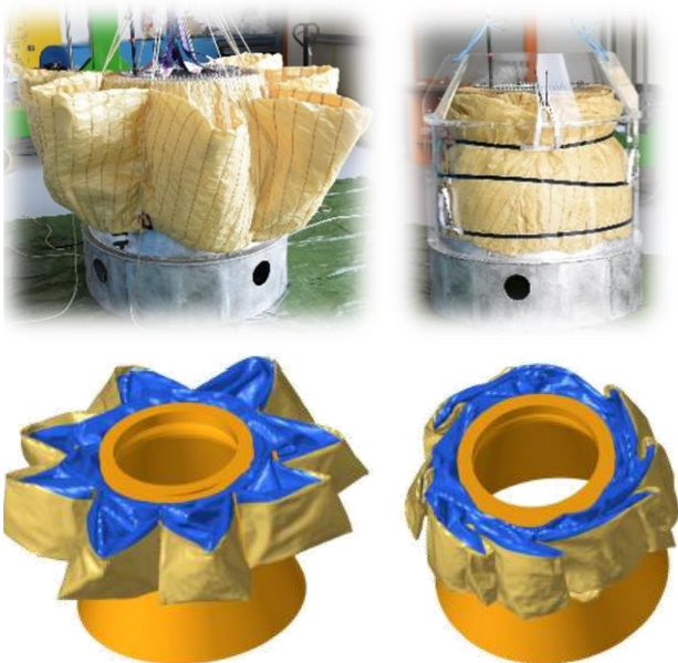
Figure 18: IS folding/stowing test and simulation
