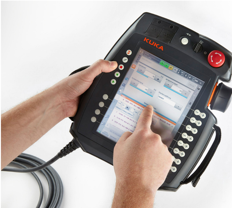
Fig. 2.1 KUKA Smart Pad (SP): the device that the operators need to use to manually control and program the robot is depicted. It consists of a touch-based graphics interface, as well as of some physical buttons and switches for safety-critical operations.
