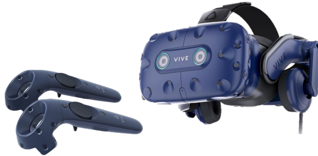
Fig. 3: HTC VIVE PRO EYE virtual reality headset with hands-held controllers.
