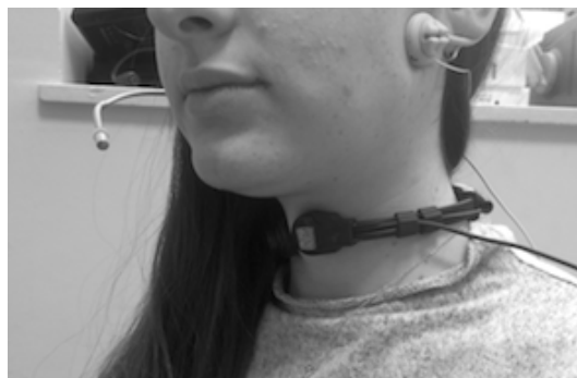
Fig. 2.1 Contact microphone and microphone in air positioning
