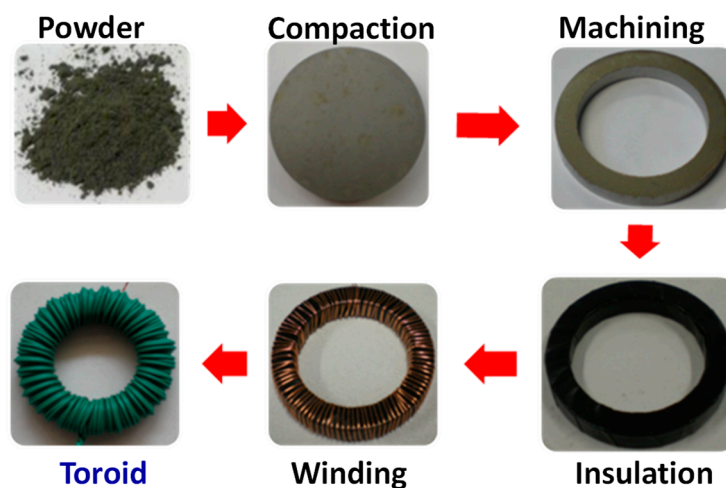
Figure 2. Different procedures of the SMC preparation specimens for magnetic characterization through a toroidal magnetic test.
