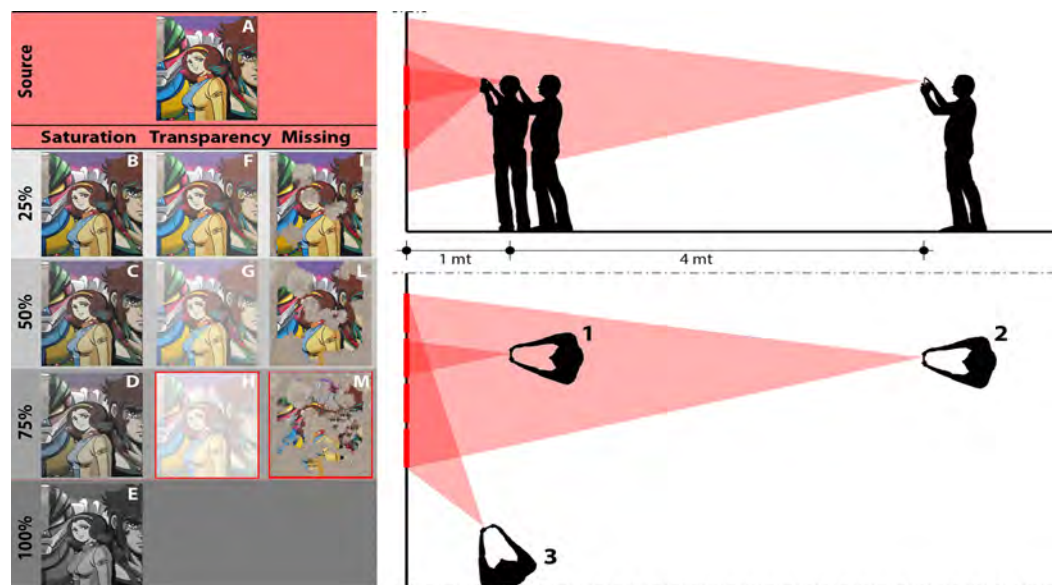
Fig. 3. Scheme of the experimentation: on the left are the different types of targets that simulate the transformation of the artwork in time; on the right, the scheme of taking in plan and elevation.
