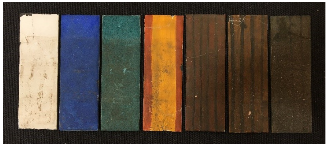
Figure 12. 5a set after cleaning tests using best conditions. Not soiled area on the top.
