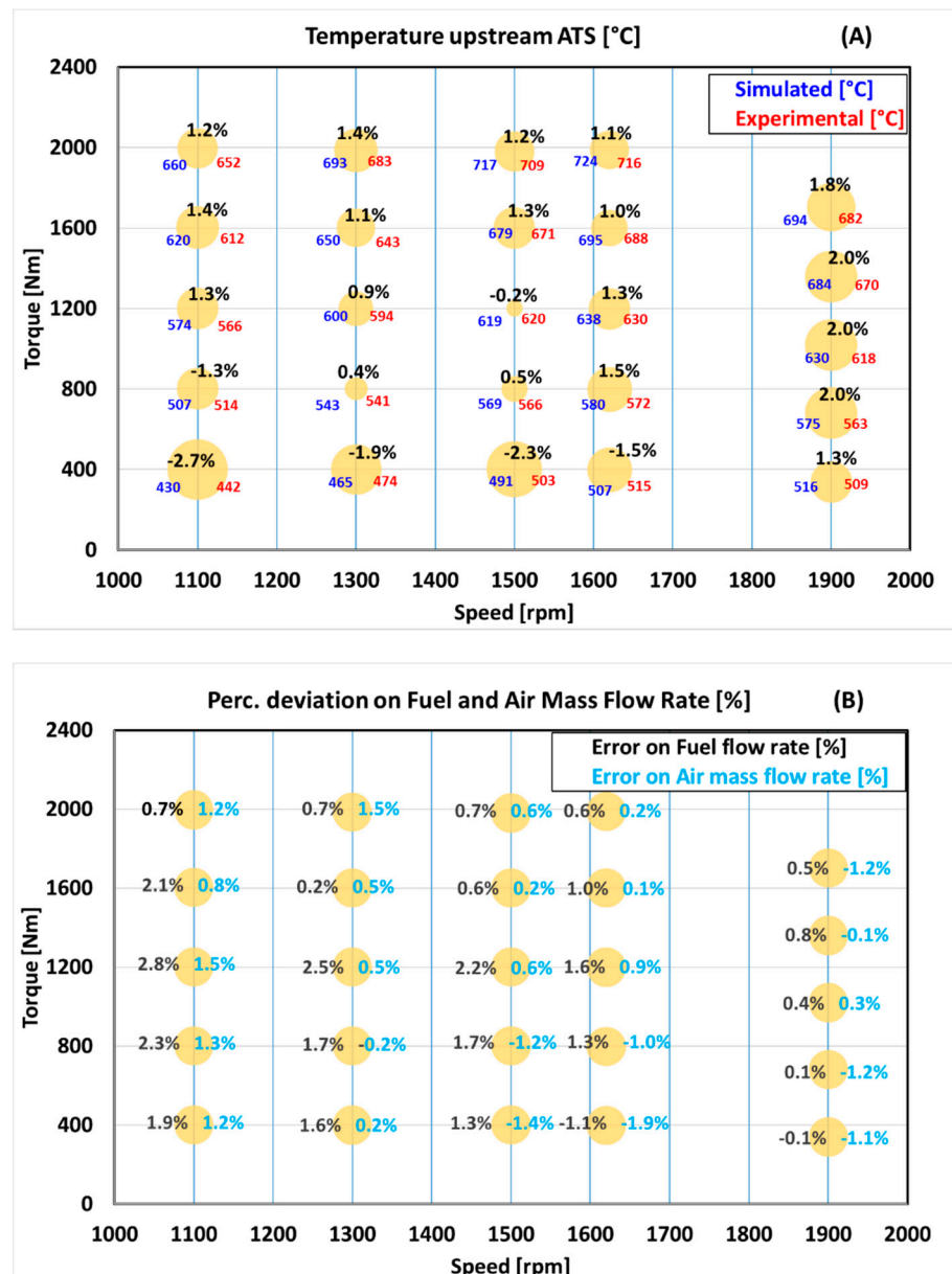
Figure 8. Percentage deviation between simulated and experimental data before ATS temperature (A); fuel and air mass flow rate (B) in the 25 tested operating conditions.
