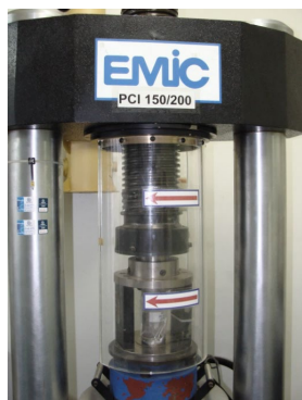
Fig. 10: Testing device used for the evaluation of the compressive strength of tailings-added geopolymer samples.
