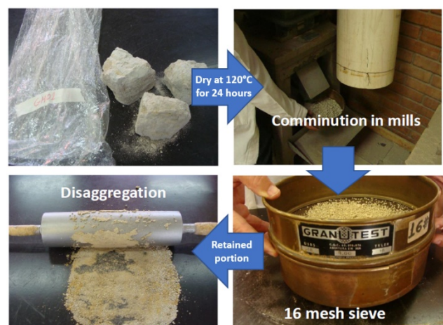
Fig. 3: Preparation method of kaolinite samples
