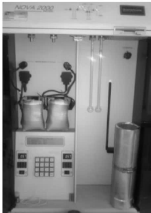
Fig. 4: Quantachrome apparatus for the specific area evaluation.
