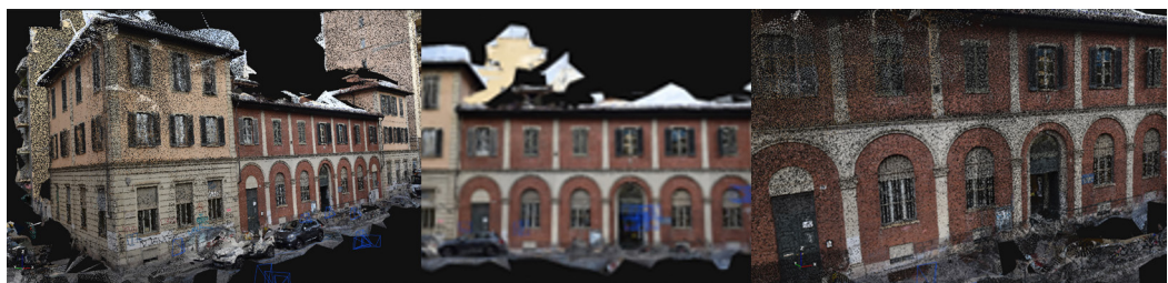
Fig. 08. Some images of the point cloud generated within the 3D Zephyr Free 5.019 software. Image by author
