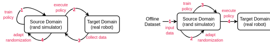
Fig. 1: Conceptual illustration of online (left) and offline (right) adaptive domain randomization.
