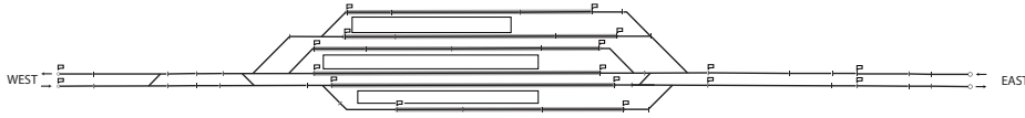
Fig. 1: A subsection of the real-world railway station considered in the experimental analysis. Flags are used to delimit itineraries; shorter segments represent track segments; bold indicates platforms.
