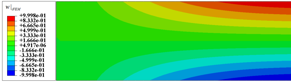
(a) Contour plot of transverse deflection for Mode 2 using CFG-D
