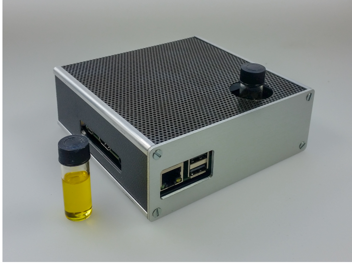
Figure 1. Photo of the fluorescence sensor an olive oil samples in the glass vials.
