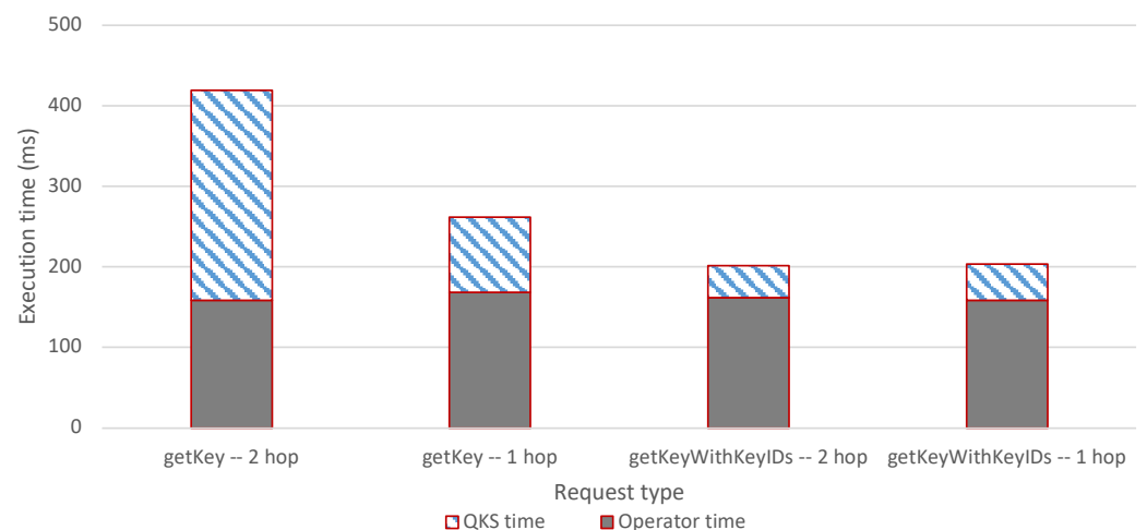
Figure 10. Execution time of the getKey and getKeyWithId functions for Point-to-Point and Multi-hop exchanges.
