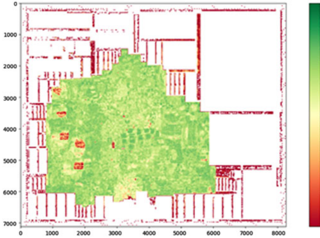
Fig. 13. Visualization over the layout of the toggle coverage produced by pseudo-random patterns used to excite the single full scan chain.
