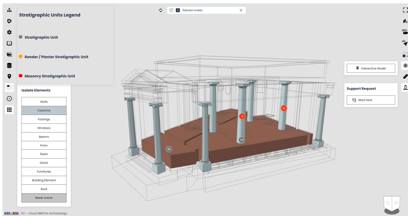
Figure 12. The Domus Regia HBIM model inside the ARK-BIM environment. Additional plugins are on the left and right side of the window: details on picked stratigraphic units and “IfcColumn” isolated in the 3D environment.
